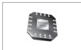
LFCSP (LeadFrame Chip Scale Package)
