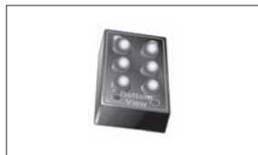
WLCSP (Wafer Level Chip Scale Package)
