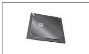
PBGA (Plastic Ball Grid Array)
